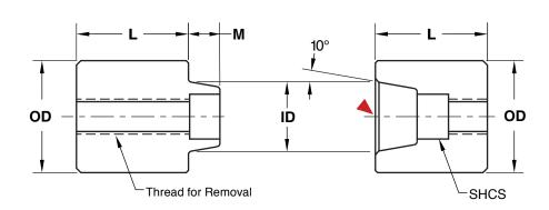
Male: M DC53 H Core: 58-62 HRC, Surface: 80 HRC S Titanium Nitride Coated
